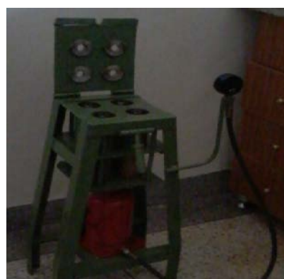
Figure 2.1: Manually operated hydraulic briquette press connected to pressure gauge
